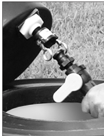
Float valve tub disconnected.
