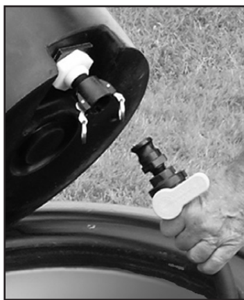
Float valve tub disconnected.
