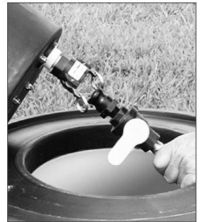
Floatless valve tub disconnected.
